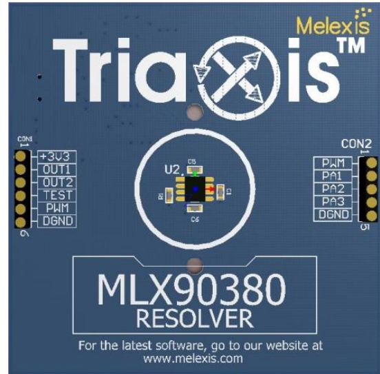
Figure 1: MLX90380 Resolver Evaluation/Demonstration board
