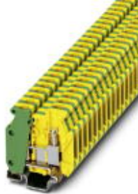
Ground modular terminal block, Connection method: Screw connection, Cross section: 0.2 mm 2 - 4 mm 2 , AWG 24 - 12, Width: 5.2 mm, Color: green-yellow, Mounting type: NS 15
