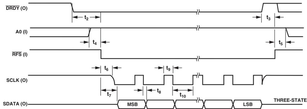
Figure 10. Self-Clocking Mode, Output Data Read Operation
