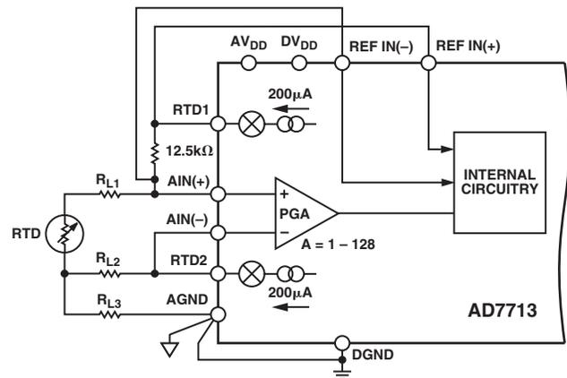
Figure 20. 3-Wire RTD Application with the AD7713
