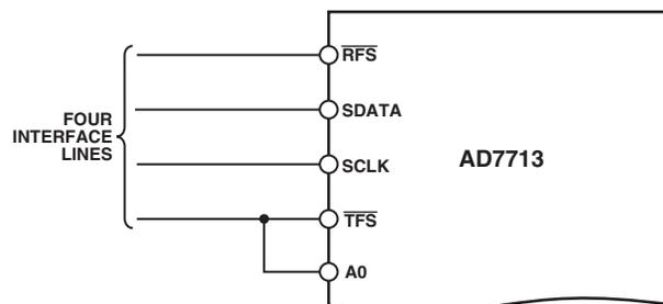
Figure 14. Simplified Interface with  $\overline{TFS}$  Connected to A0
