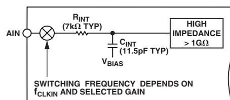
Figure 7. AIN1, AIN2 Input Impedance
