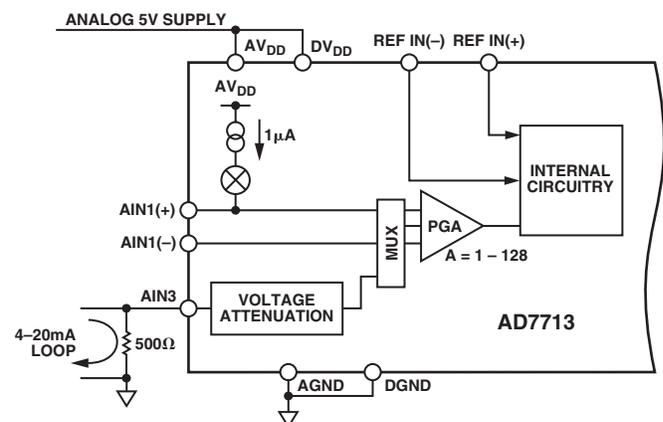
Figure 21. 4-20 mA Measurement Using the AD7713
