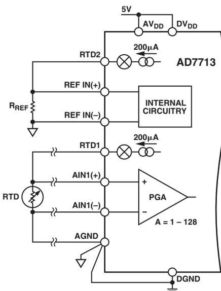
Figure 19. 4-Wire RTD Application with the AD7713
