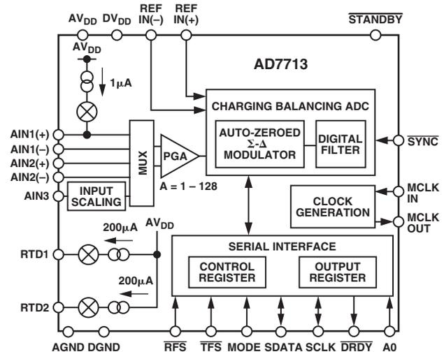
CMOS construction ensures low power dissipation, and a hardware programmable power-down mode reduces the standby power consumption to only 150 μW typical. The part is available in a 24-lead, 0.3 inch wide, PDIP and CERDIP as well as a 24-lead SOIC package.
