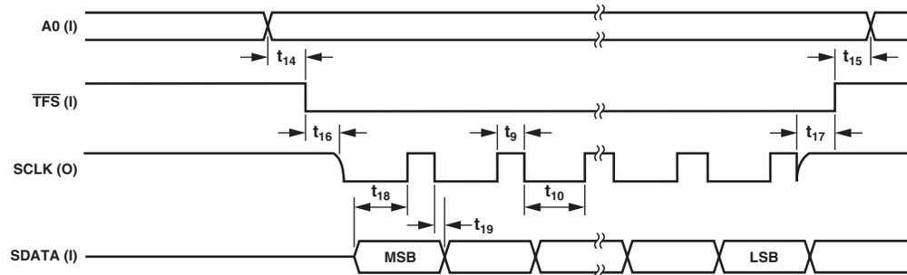
Figure 11. Self-Clocking Mode, Control/Calibration Register Write Operation
