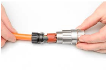
Step 15 - Push sub-assembly into shell
