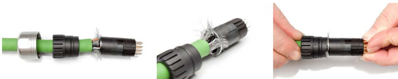
Step 10 - Position the shield as shown
