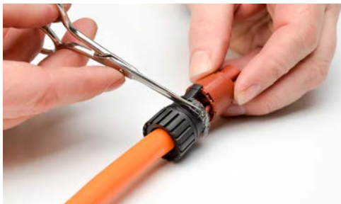
Step 14 - Trim shield as shown
