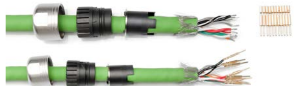
Step 6 - Crimp a contact onto each wire
