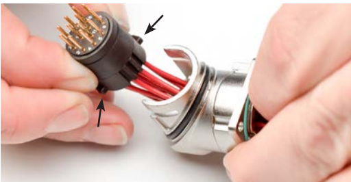
Step 5 - Locate keys on sides of insert
