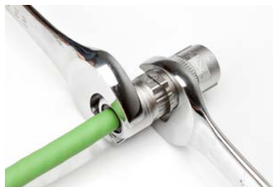
Step 16 - Tighten to 5-7 N/M using 25mm wrench
