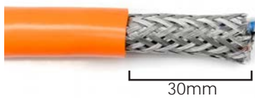
Step 1 - Remove the cable jacket 30mm
