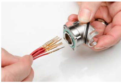
Step 3 - Slide wires through shell
