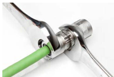
Step 16 - Tighten to 5-7 N/M using 25mm wrench
