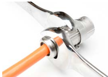
Step 17 - Tighten to 5-7 N/M using 25mm wrench
