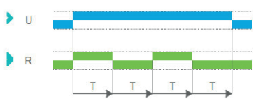
Function Di - Symmetrical flashing (ON Start)
