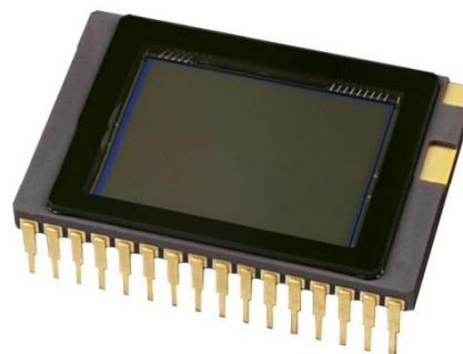
Figure 1. KAF-8300 Full Frame CCD Image Sensor
