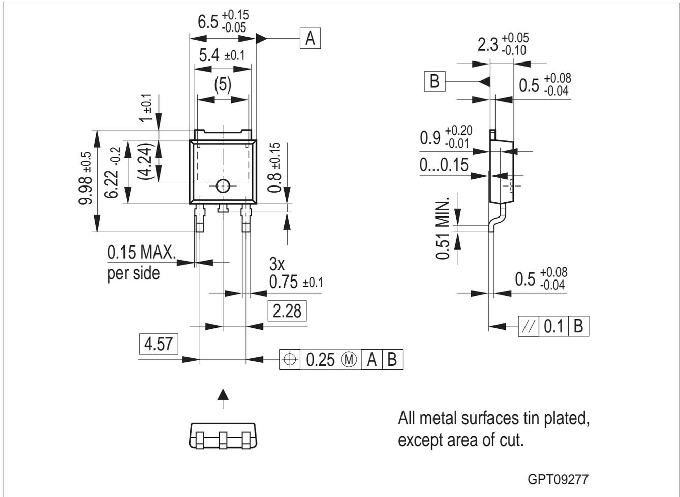
**Figure 1** PG-TO252-3-11 (Plastic Dual Small Outline Package) (RoHS-Compliant)
