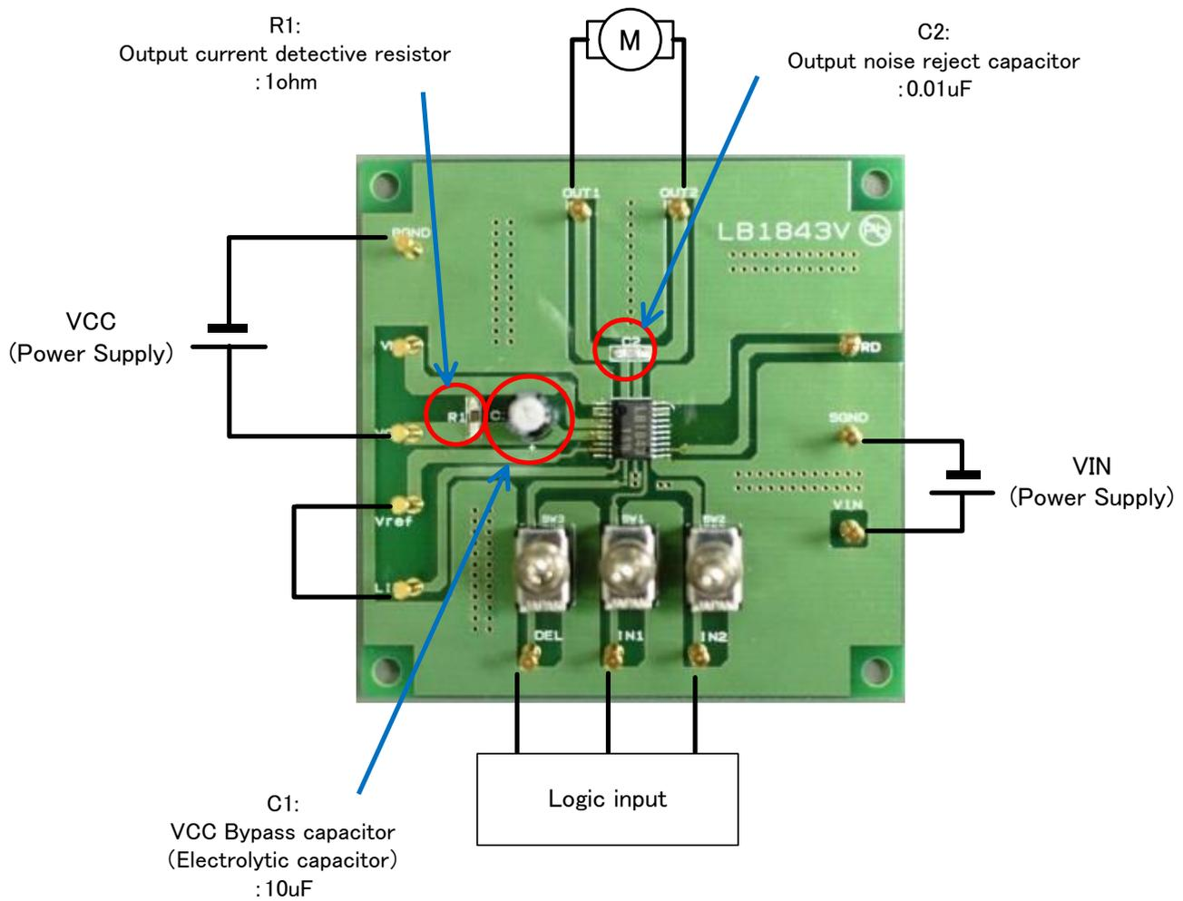
(Circuit diagram of the evaluation board)
