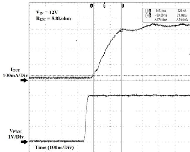
Figure 13 Output Current vs.  $V_{PWM}$  on Rising Time
