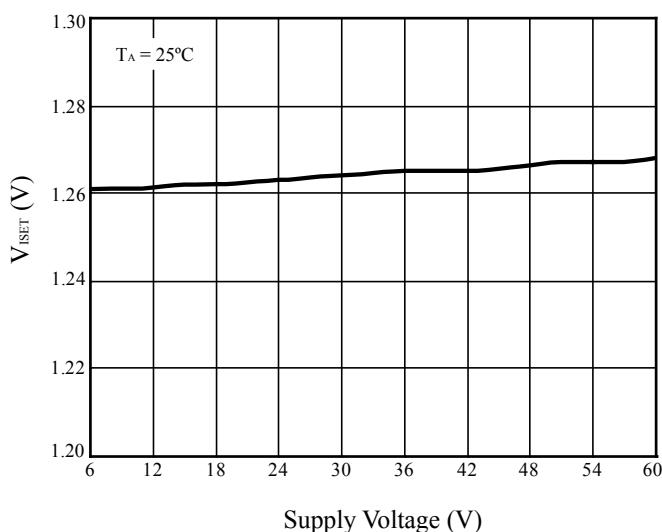
Figure 7 V<sub>ISET</sub> vs. Supply Voltage
