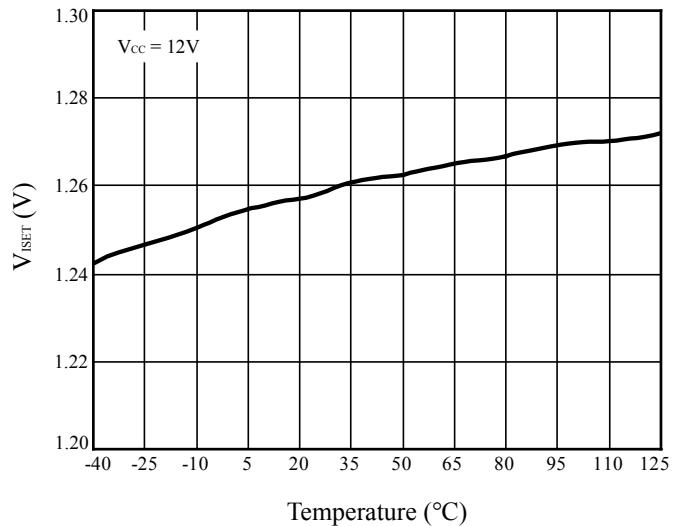
Figure 4 V<sub>ISET</sub> vs. Temperature
