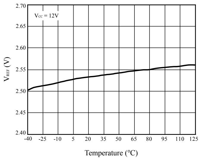
Figure 8 V<sub>REF</sub> vs. Temperature
