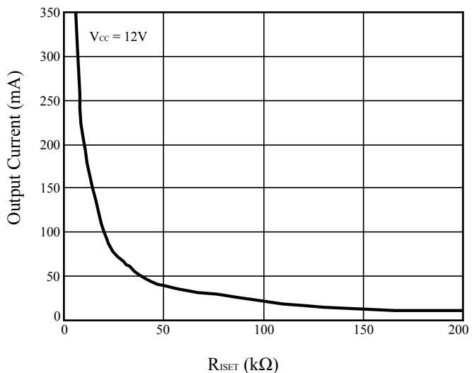
Figure 10 Output Current vs.  $R_{SET}$
