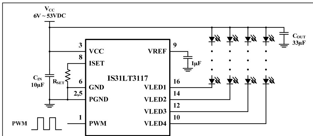
Figure 1 IS31LT3117 Directly Driving 4 LED Strings
