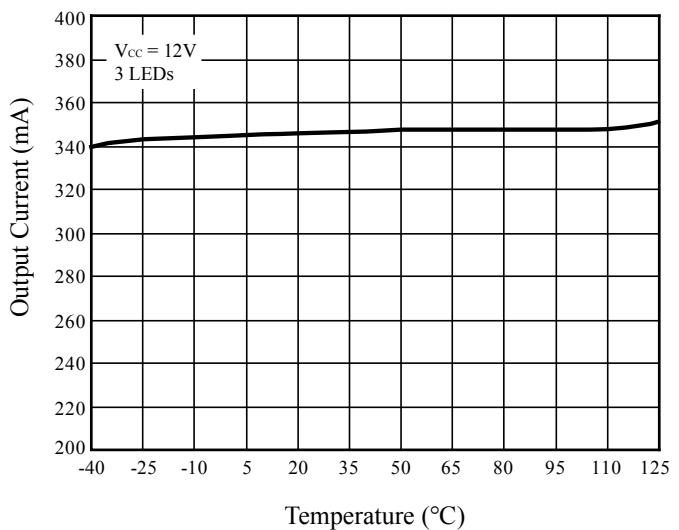
Figure 12 Output Current vs. Temperature
