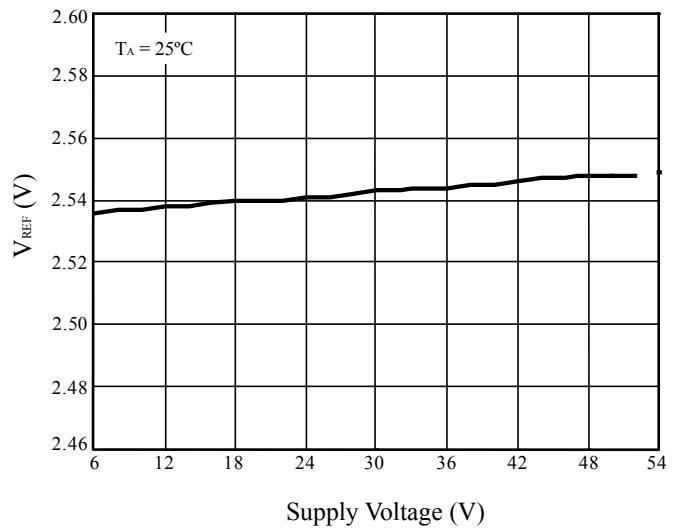
Figure 6 V<sub>REF</sub> vs. Supply Voltage
