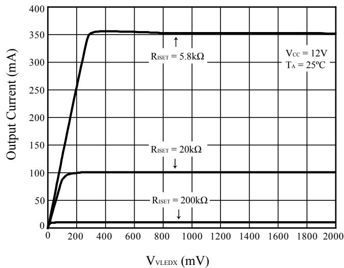
Figure 9 Output Current vs.  $V_{LEDX}$
