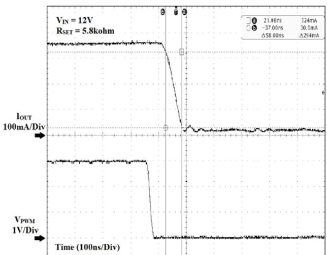
Figure 14 Output Current vs.  $V_{PWM}$  on Falling Time
