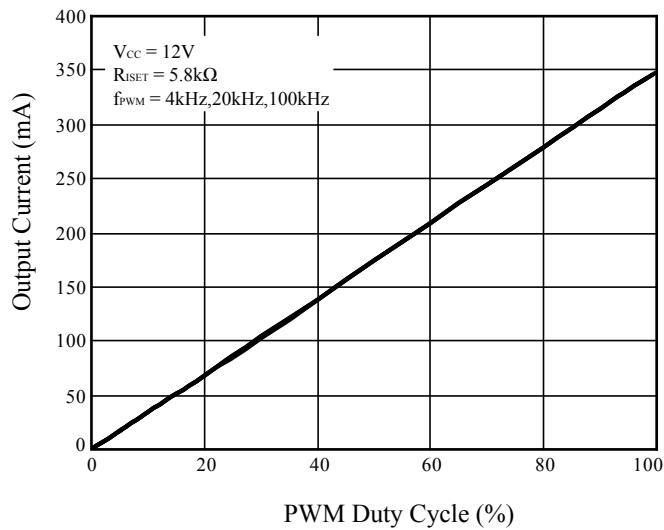
Figure 11 Output Current vs. PWM Duty Cycle
