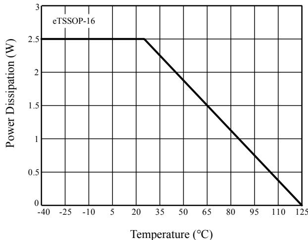
Figure 17 Dissipation curve
