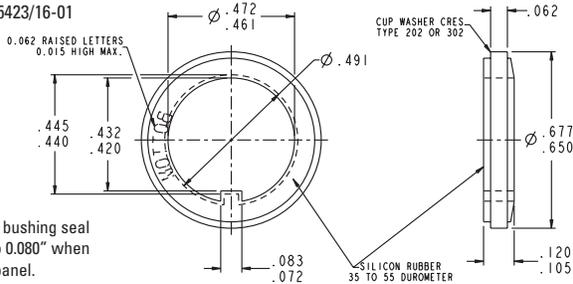
Thickness of bushing seal is reduced to 0.080" when mounted to panel.
