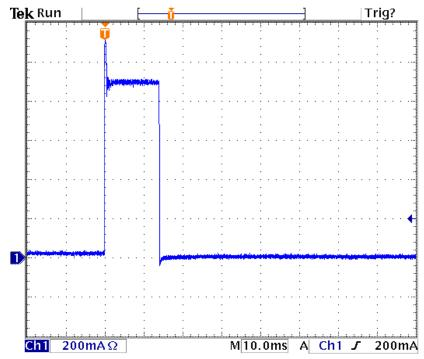
Figure 13. Overcurrent Disconnect Delay Time of 15 ms
