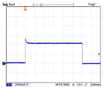
Figure 12. Overcurrent Disconnect Delay Time of 60 ms
