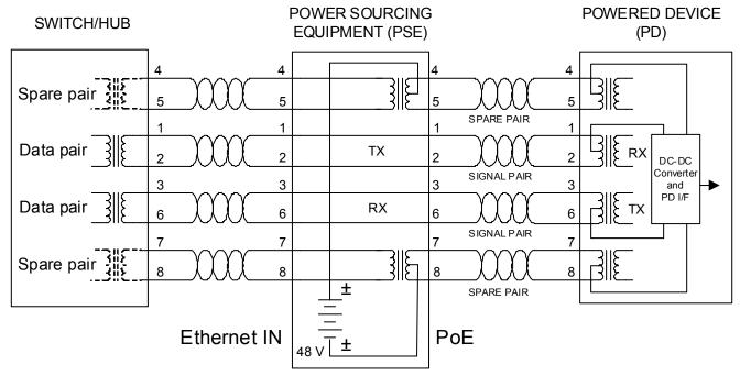
Figure 4. Midspan PSE Connection (Alternative B)\*
