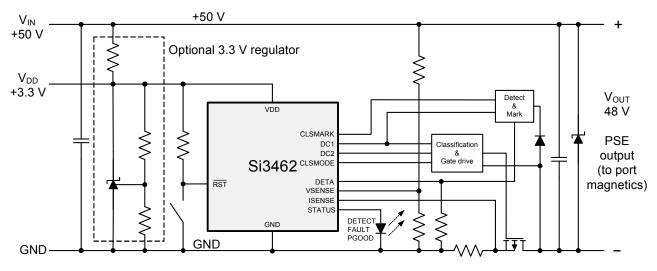
Figure 1. Typical Application Circuit (Example is for PoE; for PoE+, use +54 V nominal  $V_{\rm IN}$ )
