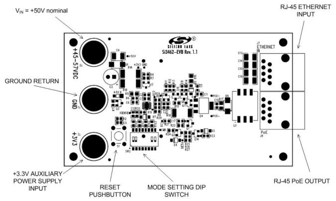
Figure 2. Placement of Connectors and Switches
