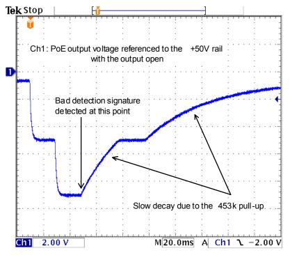
Figure 6. Detection Pulse into Open-Circuit
