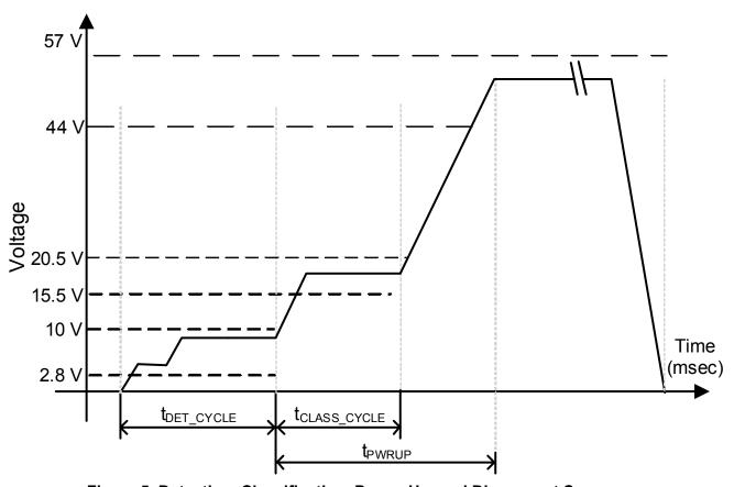
Figure 5. Detection, Classification, Power-Up, and Disconnect Sequence
