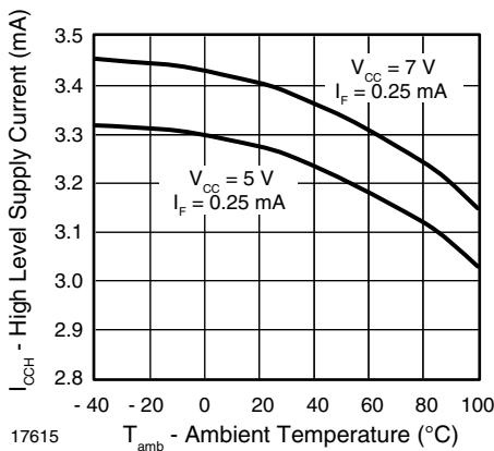
Fig. 7 - High Level Supply Current vs. Ambient Temperature
