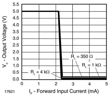
Fig. 13 - Output Voltage vs. Forward Input Current
