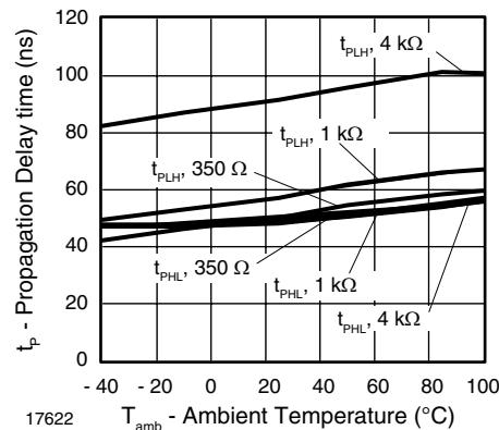
Fig. 14 - Propagation Delay vs. Ambient Temperature
