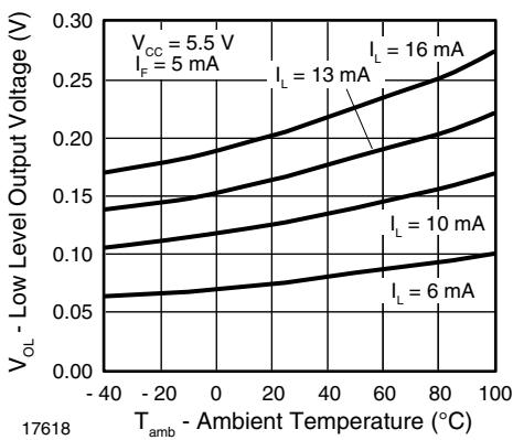
Fig. 10 - Low Level Output Voltage vs. Ambient Temperature
