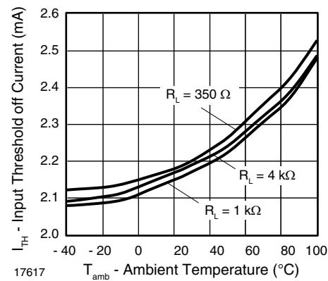
Fig. 9 - Input Threshold off Current vs. Ambient Temperature
