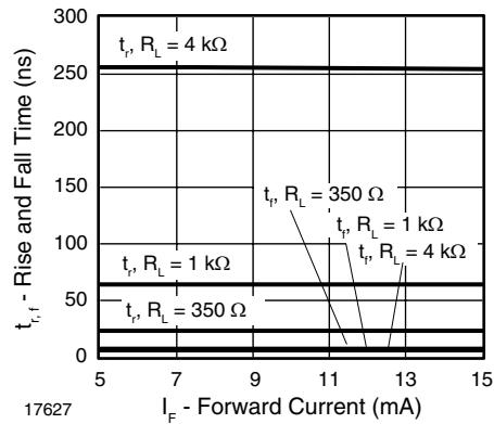
Fig. 19 - Rise and Fall Time vs. Forward Current
