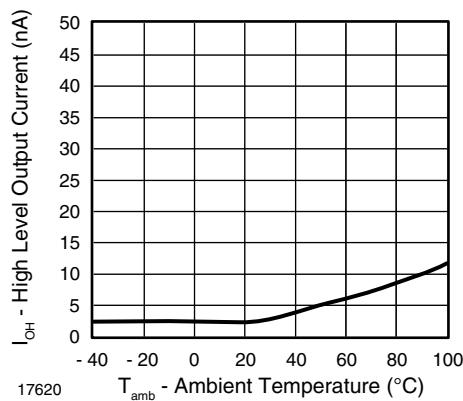
Fig. 12 - High Level Output Current vs. Ambient Temperature
