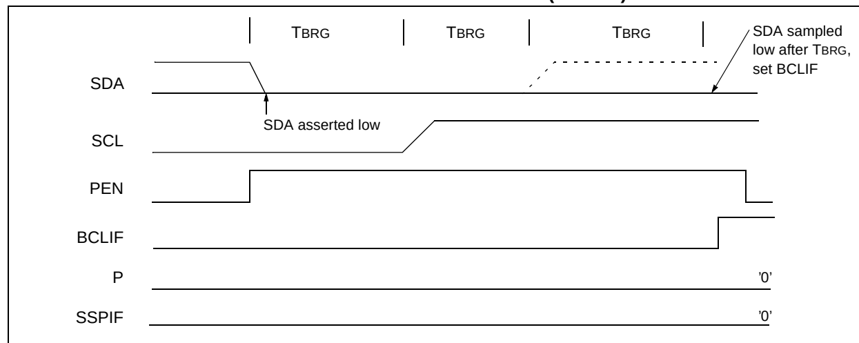
FIGURE 15-26: BUS COLLISION DURING A STOP CONDITION (CASE 1)
