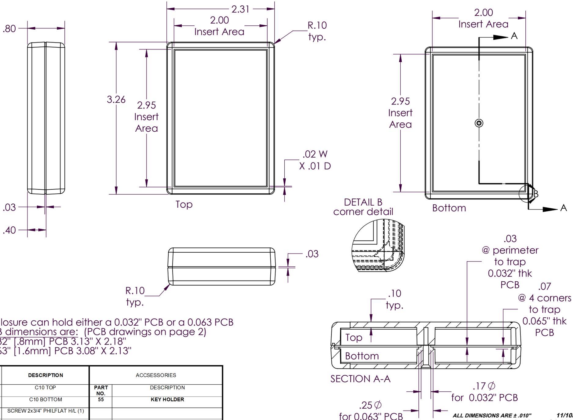
Enclosure can hold either a 0.032" PCB or a 0.063" PCB
