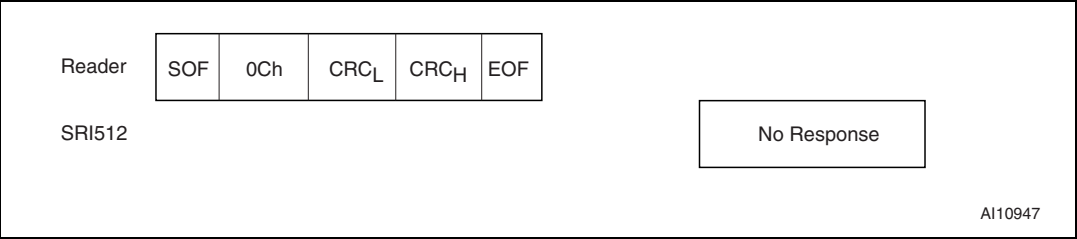
Figure 57. Reset_to_inventory frame exchange between reader and SRI512
