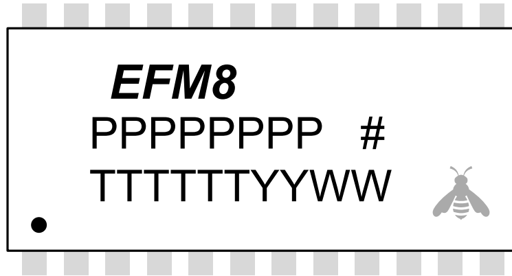
Figure 8.3. QSOP24 Package Marking
