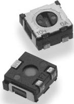
Consuming just 11.5 sq.mm of board, the 3213 has been developed specifically for a new generation of hand held equipment, where mixed technology and double sided component placement are unavoidable. These 3mm devices are just 2mm high and sealed for IR, vapour phase and full immersion wave soldering together with solvent board washing process. Also available within this range is the 3203.
