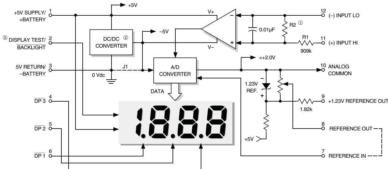
① R2 is not used on  $\pm 200mV$  (-0) models or  $\pm 2V$  (-1) models.
