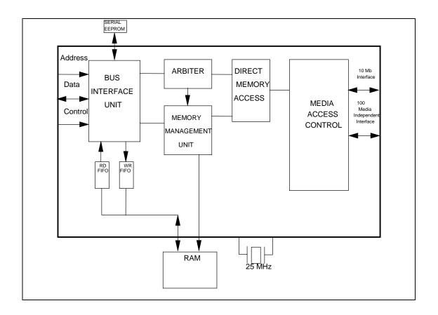
Figure 3.1 - LAN91C100FD Block Diagram
