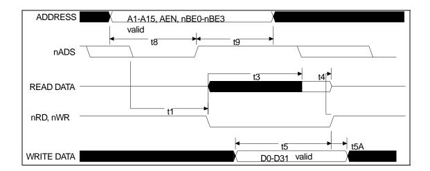
Figure 9.2 - Asynchronous Cycle - Using nADS
