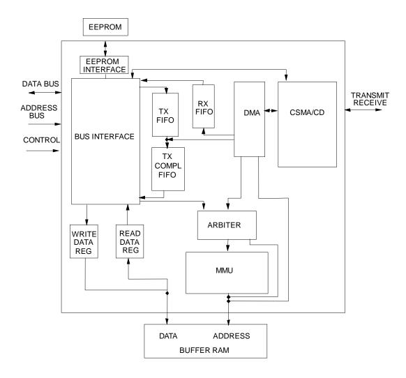
Figure 4.1 - LAN91C100FD Internal Bock Diagram with Data Path
