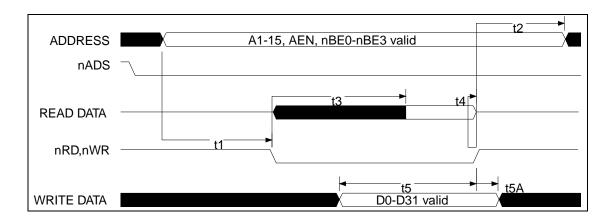
Figure 9.1 - Asynchronous Cycle - nADS=0
