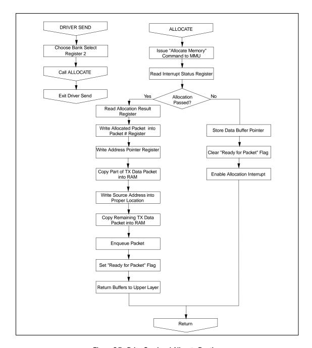
Figure 5.7 - Drive Send and Allocate Routines
