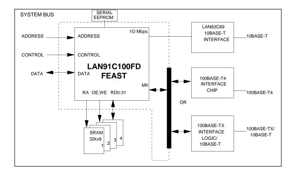
Figure 3.2 - LAN91C100FD System Diagram
