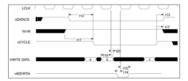
Figure 9.4 - Burst Write Cycles - nVLBUS=1
