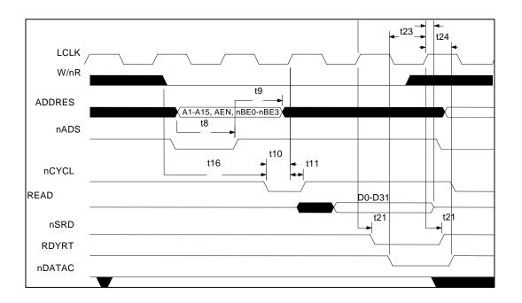
Figure 9.8 - Synchronous Read Cycle - NVLBUS=0
