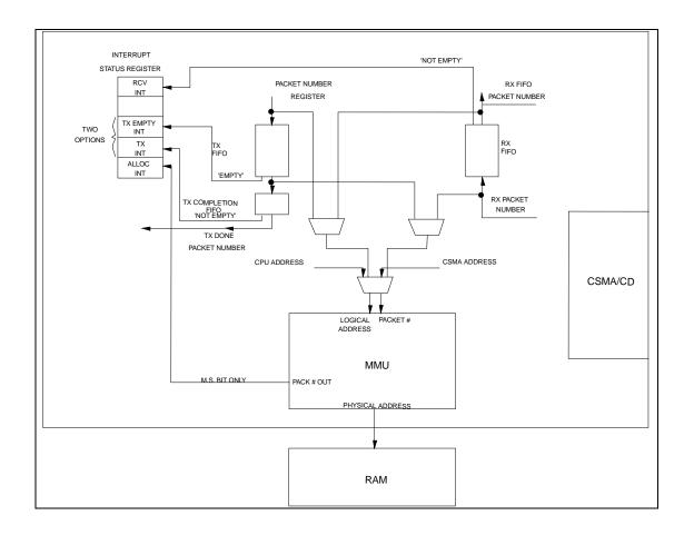
Figure 5.8 - Interrupt Generation for Transmit, Receive, MMU
