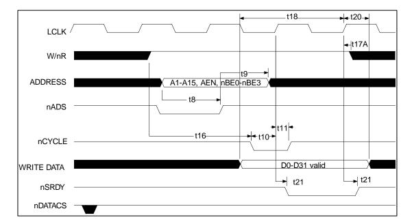
Figure 9.7 - Synchronous Write Cycles - nVLBUS=0
