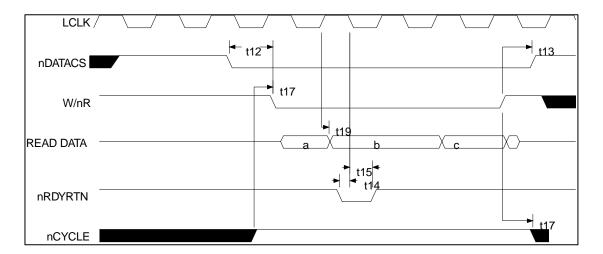
Figure 9.5 - Burst Read Cycles - nVLBUS=1
