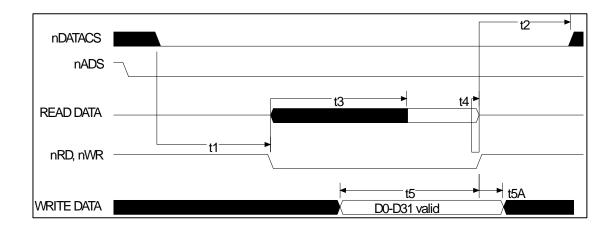
Figure 9.3 - Asynchronous Cycle - nADS=0
