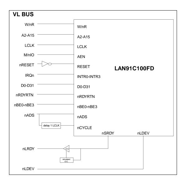
Figure 7.1 - LAN91C100FD on VL BUS
