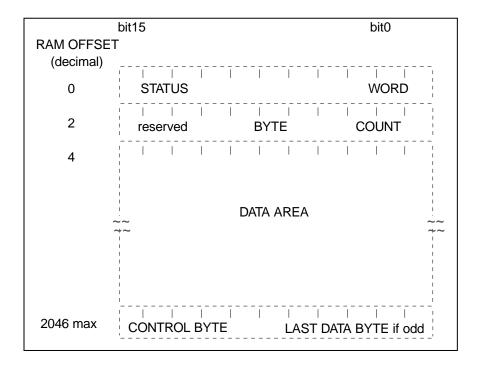
Figure 5.1 - Data Packet Format
