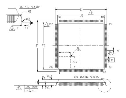
Figure 10.2 - 208 Pin TQFP Package Outlines
