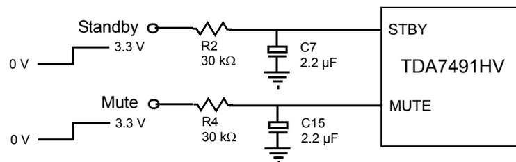
Figure 52. Turn-on/off sequence for minimizing speaker “pop”
