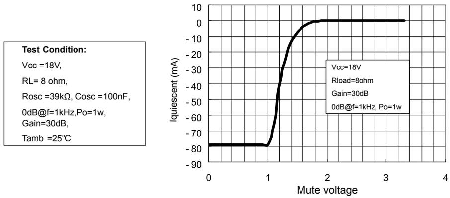
Figure 47. Current consumption vs. voltage on pin STBY
