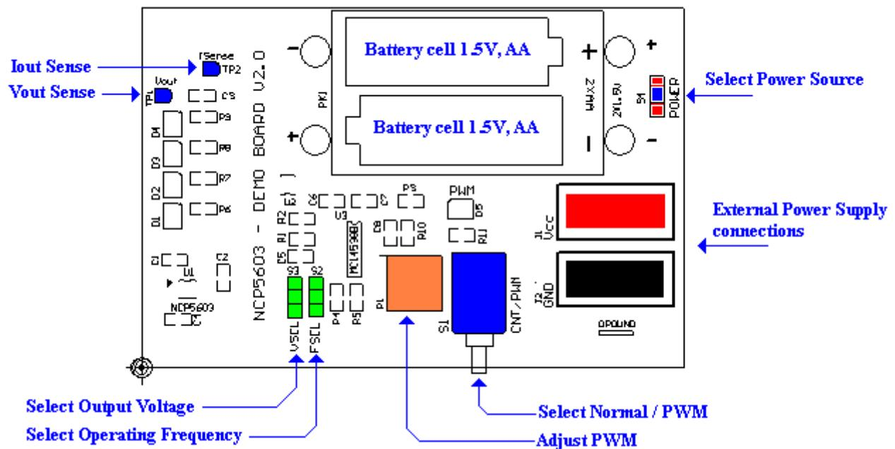
Figure 13. Evaluation Board: Silk View (Top View)
