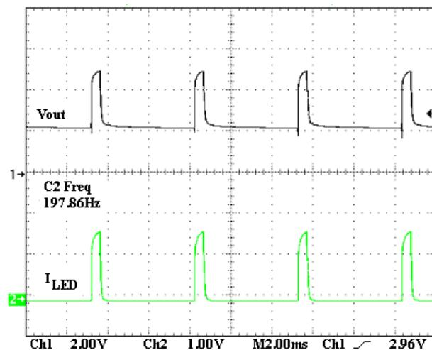
Test conditions:  $V_{bat} = 3.6$  V,  $V_{out} = 5$  V, Load = 4\*LW87S,  $I_{LED} = 25$  mA
