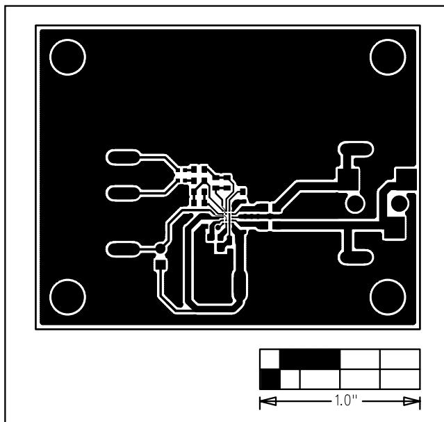
Figure 3. MAX9788 EV Kit PCB Layout—Component Side
