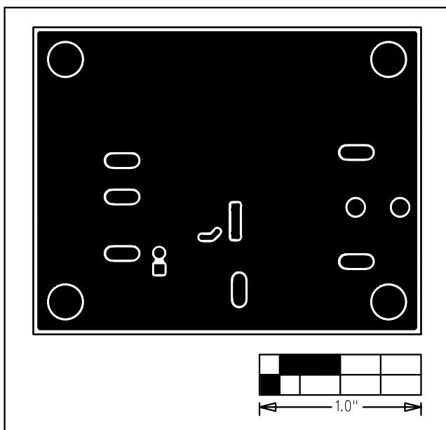
Figure 4. MAX9788 EV Kit PCB Layout—Solder Side
