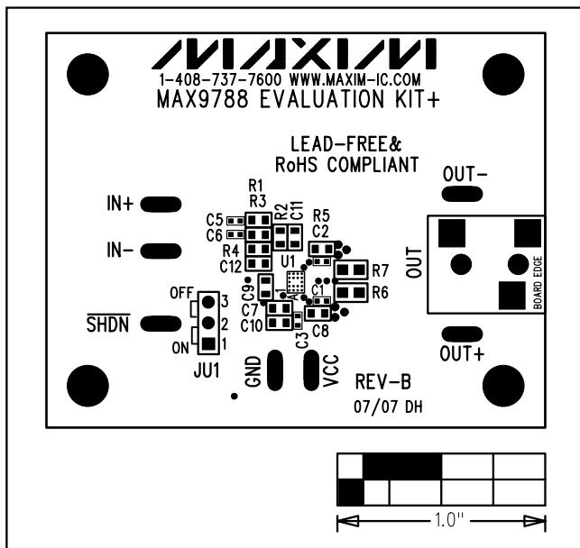
Figure 2. MAX9788 EV Kit Component Placement Guide—Component Side
