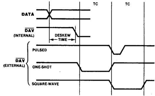
Figure 3-12. Pulsed Output Handshake Counter/Timer Duty Cycles
