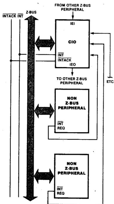
Figure 5-1. The CIO as an Interrupt Controller
