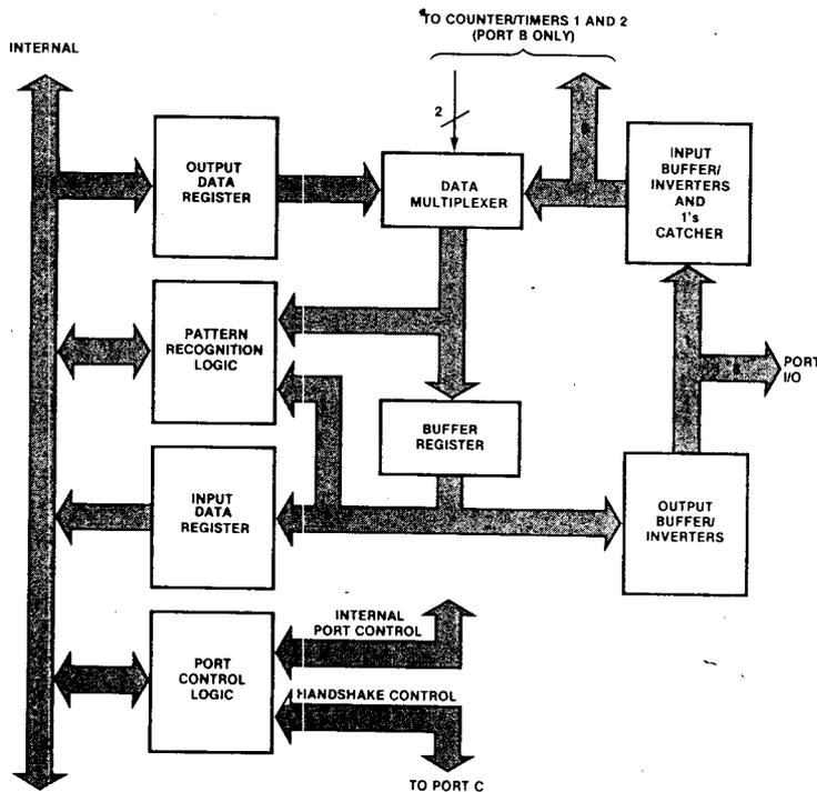
Figure 1-2. Ports A and B Block Diagram
