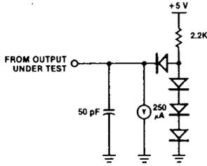
Figure 21. Standard Test Load
