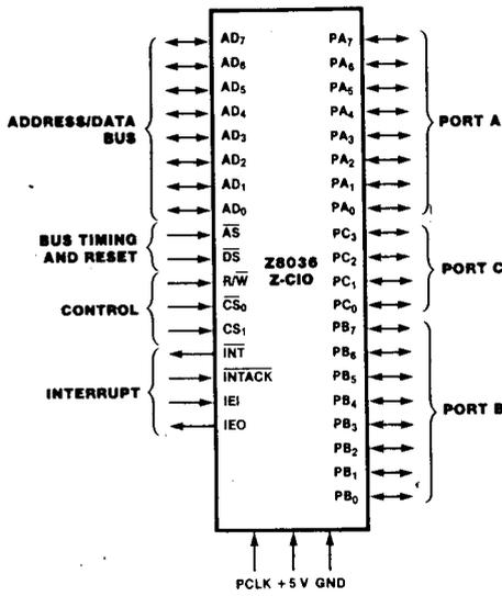
Figure 1. Pin Functions
