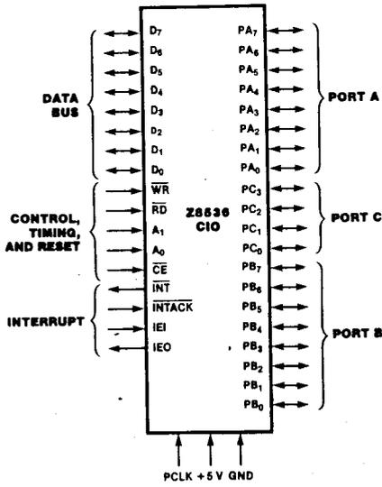
Figure 1. Pin Functions
