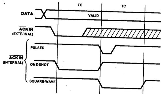
Figure 3-6. Pulsed Input Handshake Counter/Timer Duty Cycles
