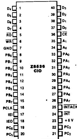
Figure 2. Pin Assignments
