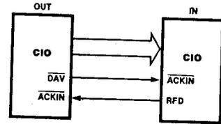
Figure 3-2. Two Interconnected CIOs Using Interlocked Handshake
