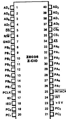
Figure 2. Pin Assignments
