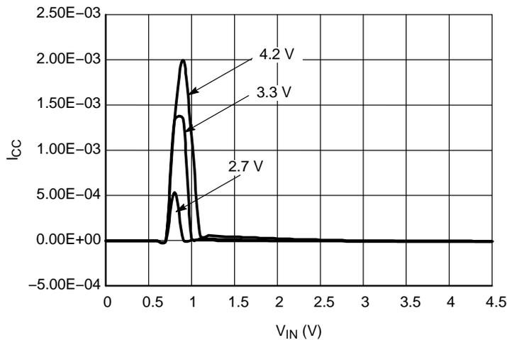
**Figure 11. I<sub>CC</sub> vs. V<sub>IN</sub>, Select Pin, All V<sub>CC</sub>'s, 25°C**
