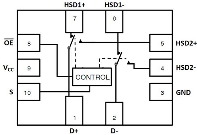
Figure 2. Pin Connections and Logic Diagram (Top View)
