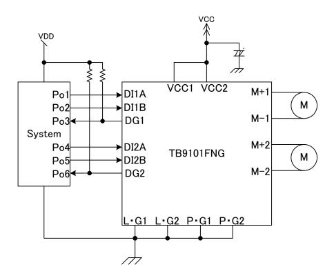
**CAUTION1**: The capacitor connected to VCC, and connect to absorb, such as voltage fluctuations due to motor load variation and noise from the outside.
