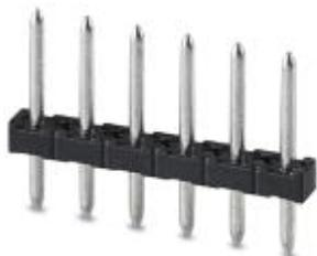
Pin strip, nominal current: 8 A, number of positions: 6, pitch: 3.5 mm, color: red, contact surface: Tin, The maximum current depends on the plug used. The lower of the two current values apply for plug and pin strip. The pin strip is made of highly temperature resistant plastic and is thus suitable for the reflow process.
