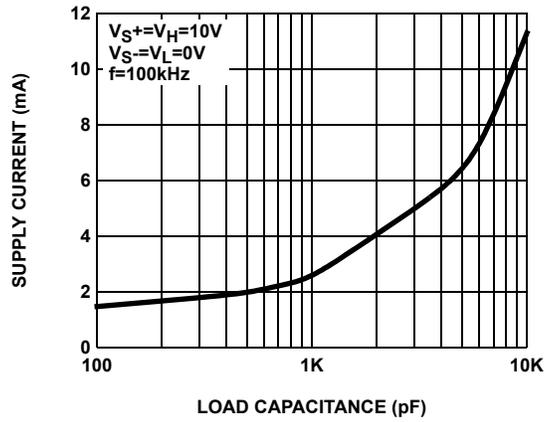
FIGURE 9. SUPPLY CURRENT PER CHANNEL vs CAPACITIVE LOAD
