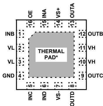
\* THERMAL PAD CONNECTED TO PIN 7 (V<sub>S-</sub>)
