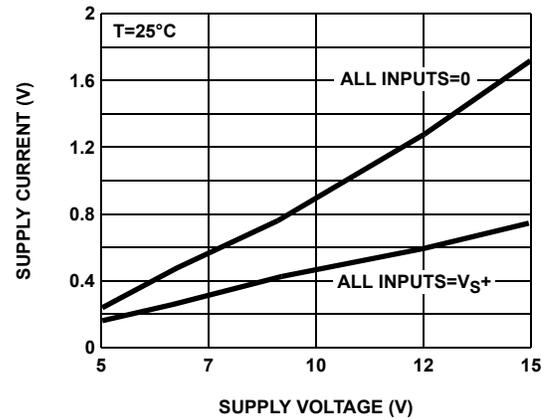
FIGURE 2. QUIESCENT SUPPLY CURRENT vs SUPPLY VOLTAGE
