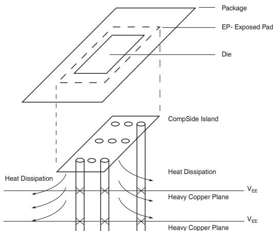
**PCB Thermal Consideration for 16-Pin QFN Package
