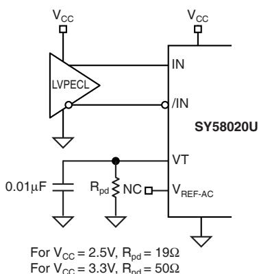
**Figure 3d. LVPECL Input Interface**
