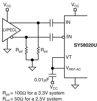
**Figure 3e. AC-Coupled LVPECL Input Interface**
