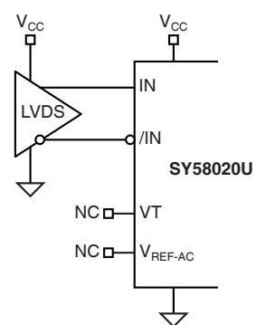
**Figure 3c. LVDS Input Interface**
