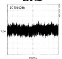
$V_{LD0}$  IS AC-COUPLED, 1mv/div  $I_{LD0} = 200 \text{mA}$   $C5 = 0.33 \mu F$
