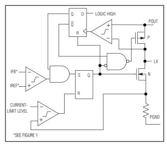
Figure 4. Controller Block Diagram in PFM Mode
