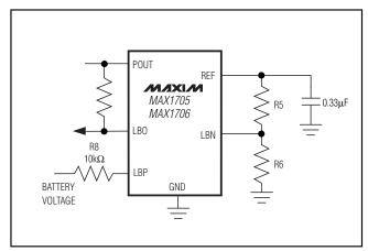
Figure 6. Detecting Battery Voltages Below 1.25V
