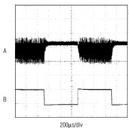
$V_{IN} = 1.2V, V_{OUT} = 3.3V$   $A = V_{OUT}, 50mV/div, 3.3V DC OFFSET$  $B = I_{OUT}, 0mA TO 200mA, 200mA/div$
