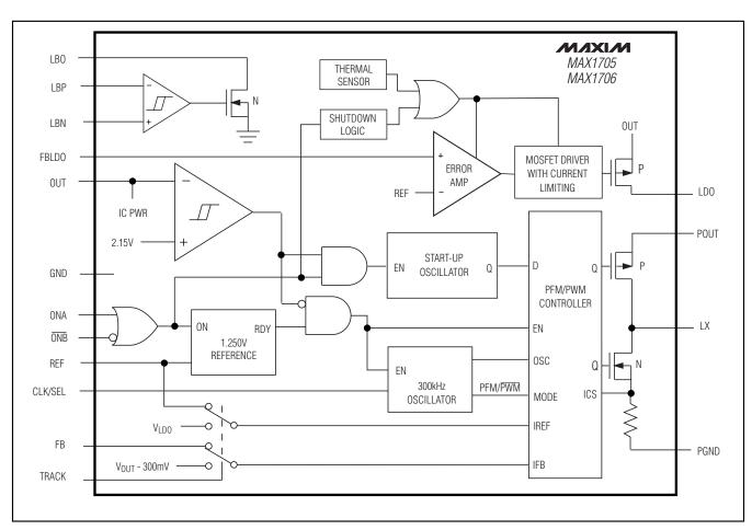
Figure 1. Functional Diagram
