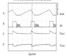
$$\begin{split} &V_{IN} = 1.2V, V_{OUT} = 4.5V, V_{LDO} = 3.3V, I_{LDO} = 40\text{mA} \\ &A = \text{INDUCTOR CURRENT, 500mA/div} \\ &B = LX VOLTAGE, 5V/div \\ &C = V_{OUT} RIPPLE, 50mV/div AC-COUPLED \\ &D = V_{LDO} RIPPLE, 5mV/div AC-COUPLED \\ &C5 = 0.33 \mu F \end{split}$$
