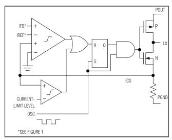
Figure 3. Simplified PWM Controller Block Diagram
