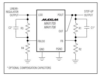
Figure 8. Feedback Connections for the MAX1705/MAX1706
