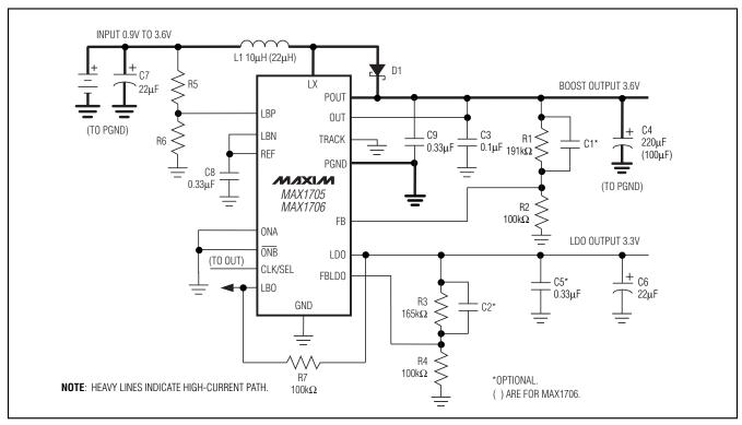
Figure 2. Typical Operating Circuit (PFM Mode)
