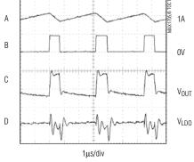
$$\begin{split} &V_{IN}=1.2V,\,V_{OUT}=4.5V,\,V_{LD0}=3.3V,\,I_{LD0}=200\text{mA}\\ &A=\text{INDUCTOR CURRENT, 500\text{mA/div}}\\ &B=LX\,\,\text{VOLTAGE, 5V/div}\\ &C=V_{OUT}\,\,\text{RIPPLE, 50m/div AC-COUPLED}\\ &D=V_{LD0}\,\,\text{RIPPLE, 5m/div AC-COUPLED}\\ &C5=0.33\mu\text{F} \end{split}$$
