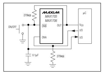
Figure 11. Momentary Pushbutton On/Off Switch
