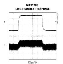
$$\begin{split} &I_{OUT} = 0 mA, \, V_{OUT} = 3.3 V \\ &A = V_{IN}, \, 1.5 V \, TO \, 2.0 V, \, 200 mV/div \\ &B = V_{OUT}, \, 10 mV/div, \, 3.3 V \, DC \, \, OFFSET \end{split} \label{eq:lower_lower}$$
