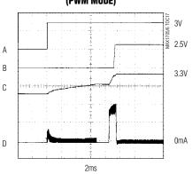
$\begin{array}{l} V_{IN}=1.2V, LOAD=1k\Omega, \ \overline{ONB} \ TIED \ TO \ OUT \\ A=ONA, 2V/div \\ B=V_{LDO}, 2V/div \\ C=V_{OUT}, 2V/div \\ D=INDUCTOR \ CURRENT, 500mA/div \end{array}$
