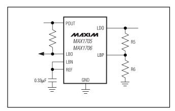
Figure 5. Using the Low-Battery Comparator to Sense the Output Voltage
