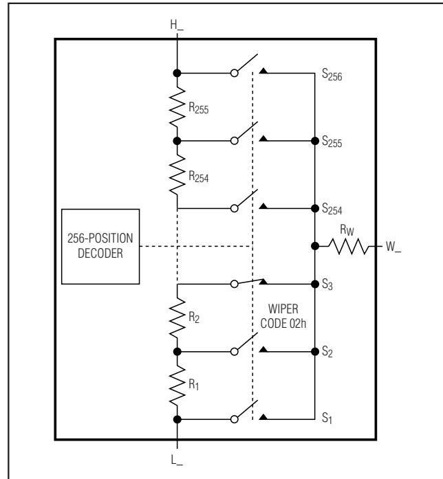
Figure 2. Potentiometer Configuration
