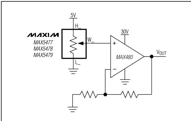
Figure 9. Positive LCD Bias Control Using a Voltage-Divider
