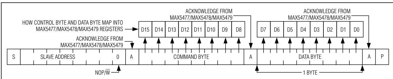
Figure 8. Command and Single Data Byte Received
