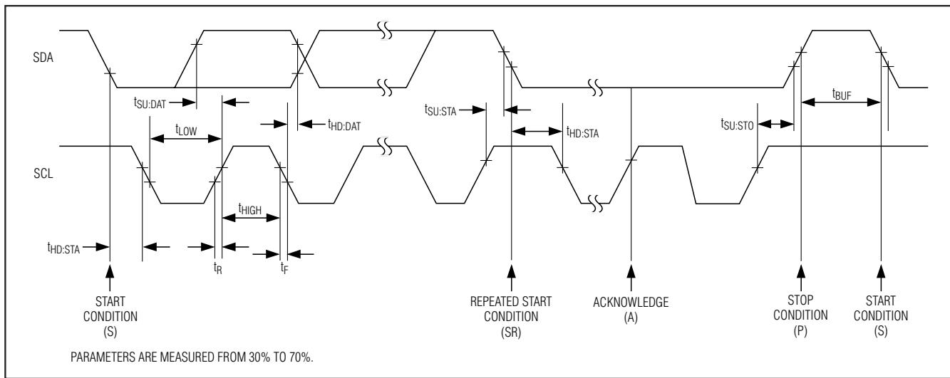
Figure 1. I<sup>2</sup>C Serial-Interface Timing Diagram
