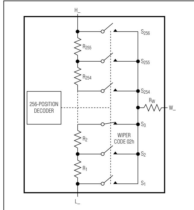
Figure 2. Potentiometer Configuration
