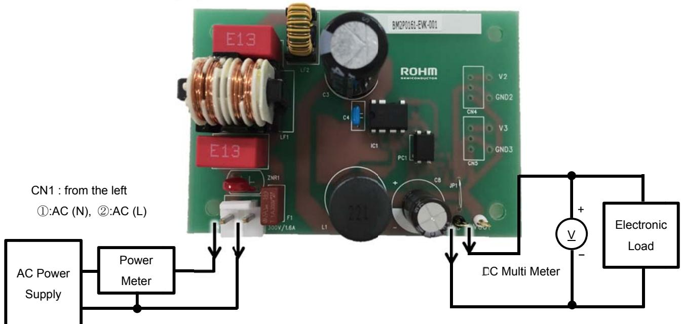
Figure 1. Connection Circuit
