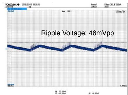
Figure 15. V<sub>OUT</sub> Ripple Voltage.1
