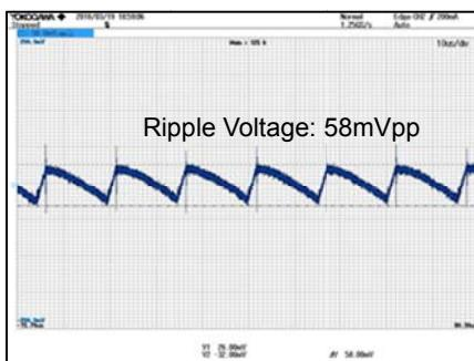
Figure 17. V<sub>OUT</sub> Ripple Voltage.3
