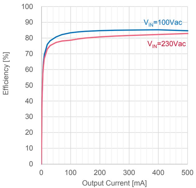
Figure 7. LOAD Regulation ( $I_{OUT}$  vs. Efficiency)Table 2. Load Regulation ( $V_{IN}=100\text{Vac}$ )Table 3. Load Regulation ( $V_{IN}=230\text{Vac}$ )
