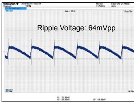
Figure 20. V<sub>OUT</sub> Ripple Voltage.6
