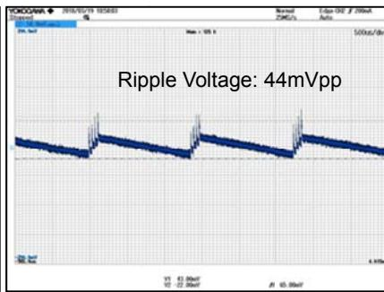
Figure 19. V<sub>OUT</sub> Ripple Voltage.5
