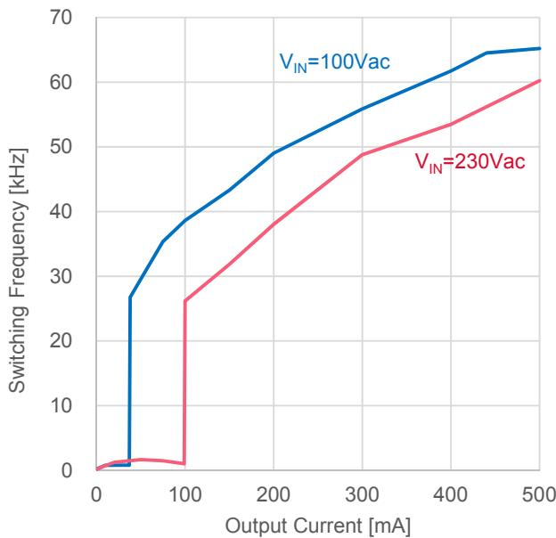
Figure 12. Switching Frequency ( $I_{OUT}$  vs.  $F_{sw}$ )• Coil Peak Current
