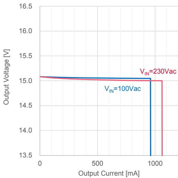
Figure 6. Load Regulation ( $I_{OUT}$  vs.  $V_{OUT}$ )
