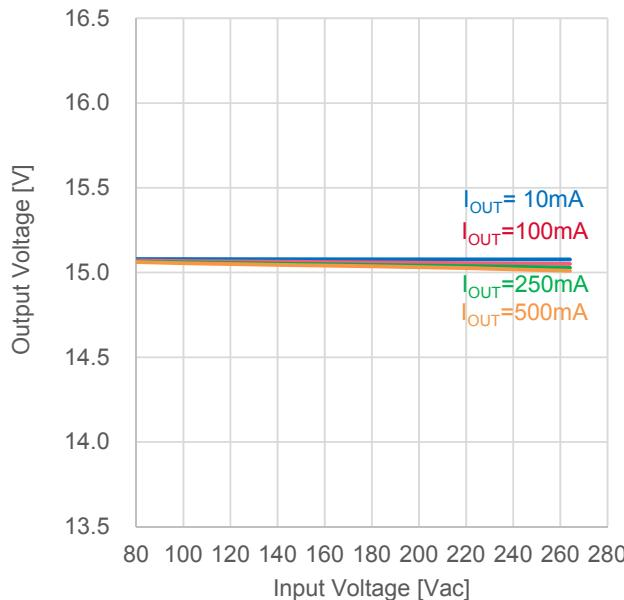
Figure 10. LINE Regulation ( $I_{OUT}$  vs.  $V_{OUT}$ )
