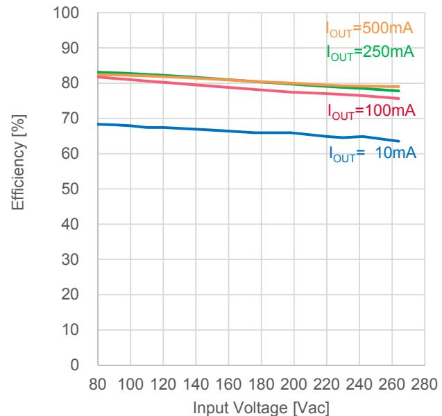
Figure 11. LINE Regulation ( $I_{OUT}$  vs. Efficiency)
