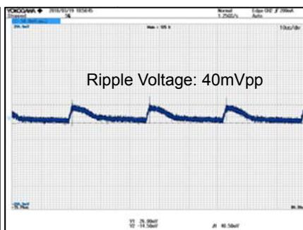
Figure 16. V<sub>OUT</sub> Ripple Voltage.2
