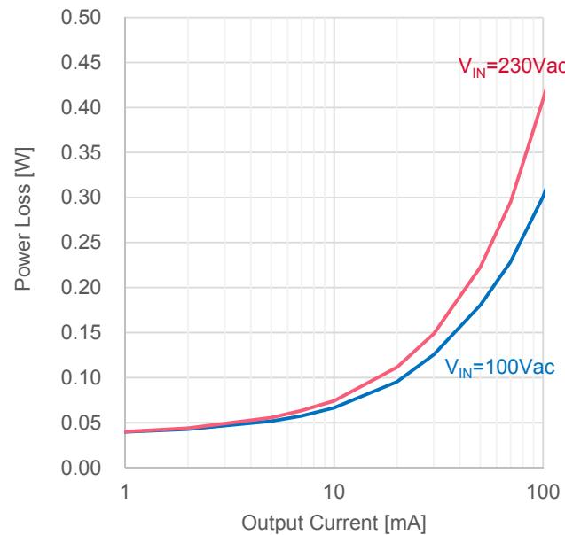
Figure 9. LOAD Regulation ( $I_{OUT}$  vs.  $P_{LOSS}$ )
