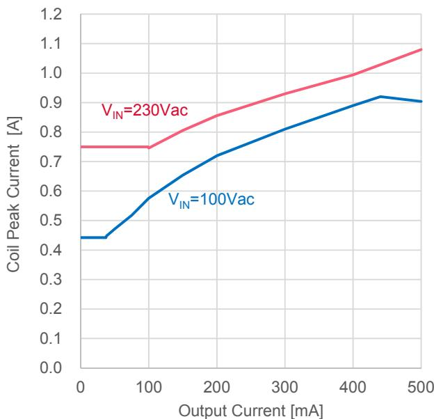
Figure 13. Coil Peak Current ( $I_{OUT}$  vs.  $I_{peak}$ )
