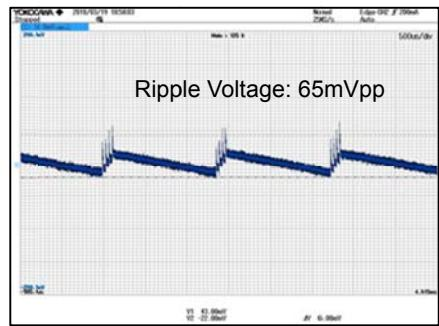
Figure 18. V<sub>OUT</sub> Ripple Voltage.4
