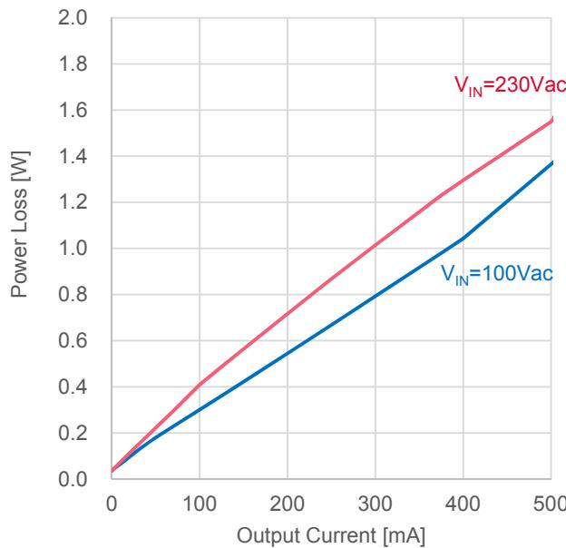
Figure 8. Load Regulation ( $I_{OUT}$  vs.  $P_{LOSS}$ )
