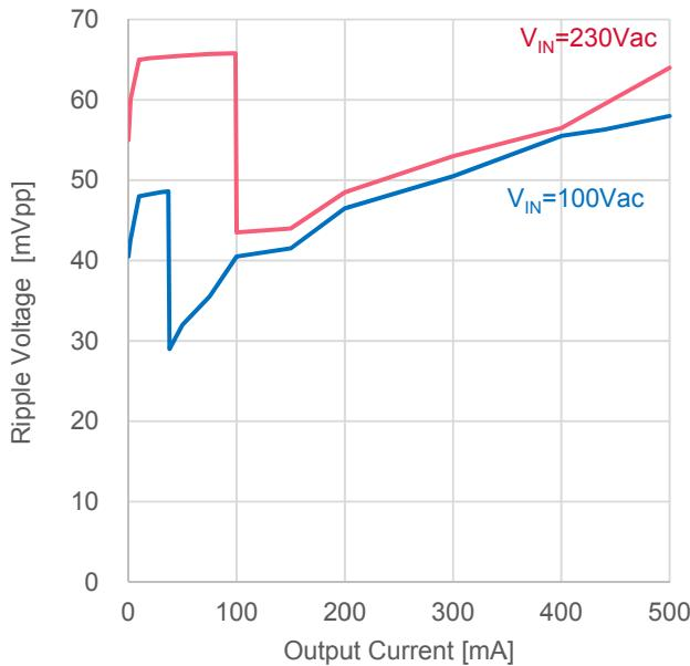
Figure 14. V<sub>OUT</sub> Ripple Voltage ( $I_{OUT}$  vs.  $V_{ripple}$ )
