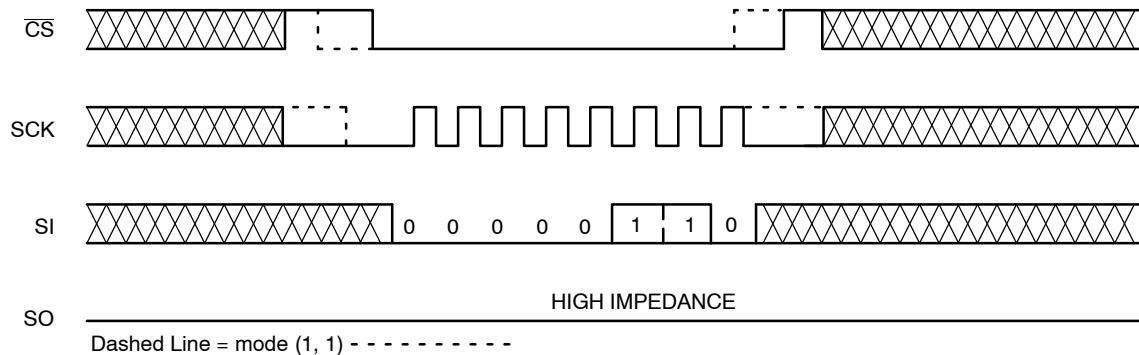
**Figure 3. WREN Timing**
