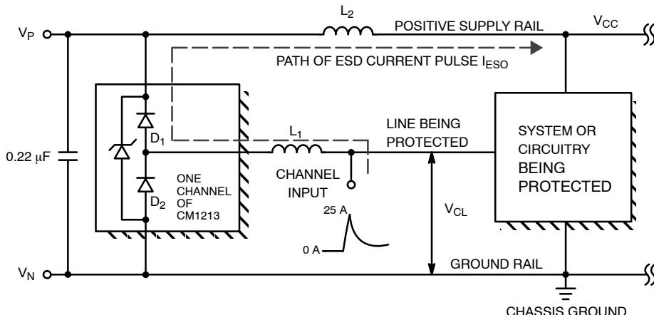
**Figure 5. Application of Positive ESD Pulse between Input Channel and Ground**
