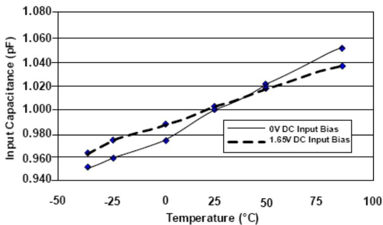
**Figure 2. Typical Variation of  $C_{IN}$  vs. Temp**
