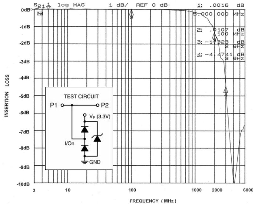
**Figure 3. Insertion Loss (S<sub>21</sub>) vs. Frequency (0 V DC Bias, V<sub>P</sub>=3.3 V)**
