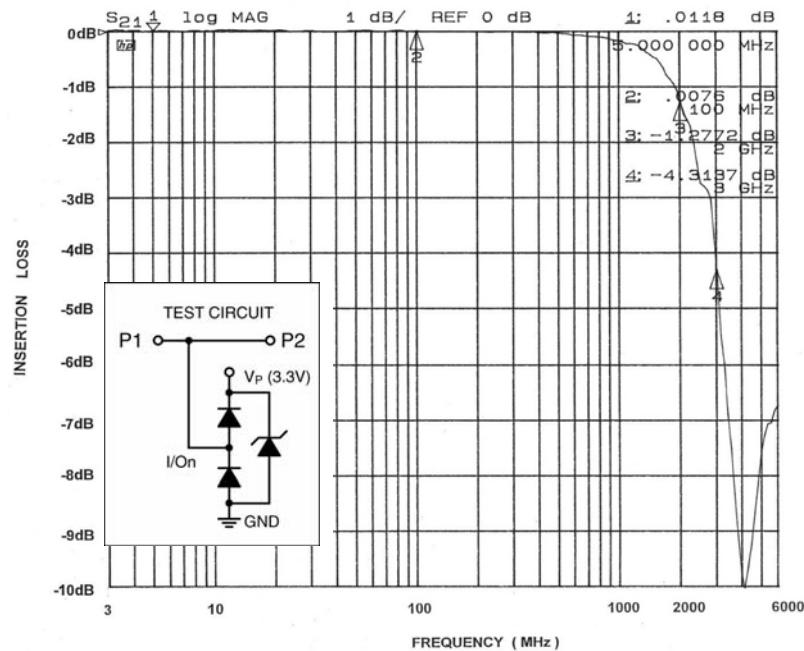
**Figure 4. Insertion Loss (S<sub>21</sub>) vs. Frequency (2.5 V DC Bias, V<sub>P</sub>=3.3 V)**
