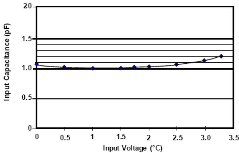
**Figure 1. Typical Variation of  $C_{IN}$  vs.  $V_{IN}$**
