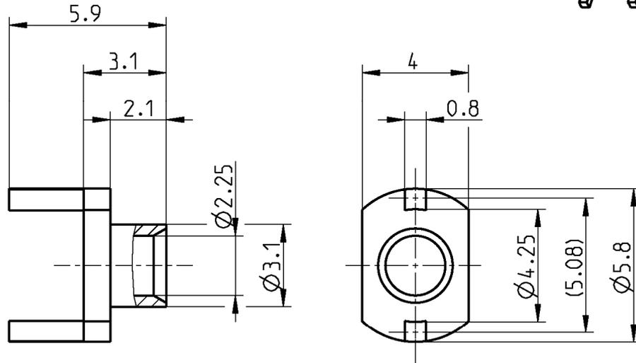
All dimensions are in mm; tolerances acc. ISO 2768 m-H
