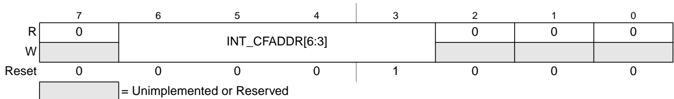
Figure 4-4. Interrupt Configuration Address Register (INT_CFADDR)
