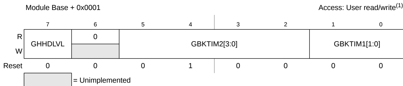
Figure 17-4. GDU Control Register (GDUCTR)
