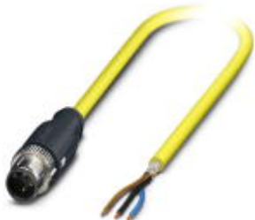
Sensor/Actuator cable, 3-position, PVC, Variable cable type, Yellow RAL 1021, shielded, Plug straight M12-SPEEDCON, A-coded, on Free cable end, Cable length: 2 m
