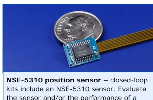
**NSE-5310 position sensor** – closed-loop kits include an NSE-5310 sensor. Evaluate the sensor and/or the performance of a closed-loop SQUIGGLE motor system.
