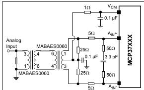
FIGURE 4-3: Transformer Coupled Input Configuration.
