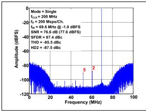
**FIGURE 3-19:** FFT for 69.6 MHz Input Signal with NSR enabled: NSR = 52,  $f_S = 200 \text{ Msps/Ch.}$ ,  $A_{IN} = -1 \text{ dBFS}$ .
