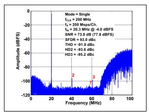
**FIGURE 3-18:** FFT for 20.3 MHz Input Signal with NSR enabled: NSR = 27,  $f_S = 200 \text{ Msps/Ch.}$ ,  $A_{IN} = -4 \text{ dBFS}$ .
