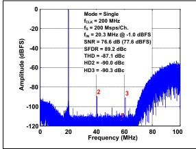
FIGURE 3-15: FFT for 20.3 MHz Input Signal with NSR enabled: NSR = 27,  $f_S = 200 \text{ Msps/Ch.}$ ,  $A_{IN} = -1 \text{ dBFS.}$
