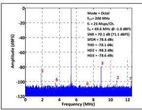
**FIGURE 3-13:** FFT for 69.6 MHz Input Signal:  $f_S = 25$  Msps/Ch., Octal,  $A_{IN} = -1$  dBFS.
