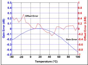
**FIGURE 3-40:** Gain and Offset Error Drifts vs. Temperature Using Internal Reference, with Respect to  $25^{\circ}$ C:  $f_S = 200$  Msps.
