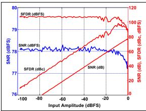
**FIGURE 3-29:** SNR/SFDR vs. Analog Input Amplitude:  $f_S = 200$  Msps,  $f_{IN} = 70$  MHz, High-Reference Mode (SENSE =  $AV_{DD12}$ ) with NSR enabled.  $A_{IN} \le 0.8$  dBFS for NSR.
