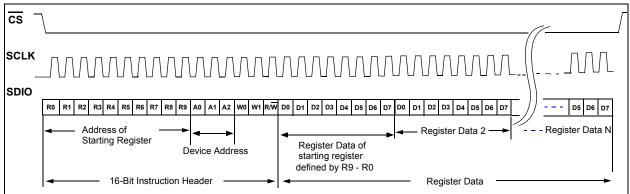
FIGURE 5-2: SPI Serial Data Communication Protocol - with LSb-First. See Figures 2-3 and 2-4 for Timing Specifications.
