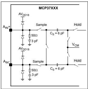
FIGURE 4-2: Equivalent Input Circuit.
