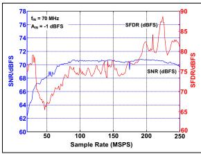
**FIGURE 3-30:** SNR/SFDR vs. Sample Rate (Msps):  $f_{IN} = 70 \text{ MHz}$ .
