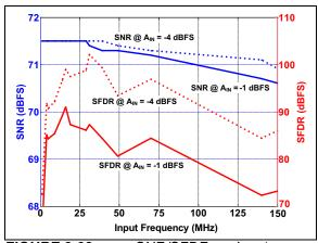
FIGURE 3-32: SNR/SFDR vs. Input Frequency.
