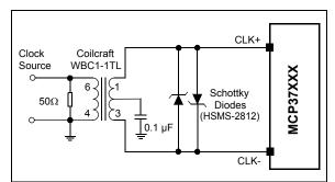
FIGURE 4-9: Transformer-Coupled Differential Clock Input Configuration.
