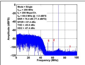
FIGURE 3-14: FFT for 69.6 MHz Input Signal with NSR enabled: NSR = 20,  $f_S = 200 \text{ Msps/Ch.}$ ,  $A_{IN} = -1 \text{ dBFS.}$
