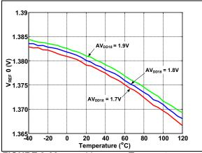
FIGURE 3-39: V<sub>REF0</sub> vs. Temperature.
