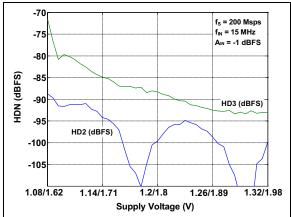
**FIGURE 3-38:** HD2/HD3 vs. Supply Voltage:  $f_S = 200 \text{ Msps}$ ,  $f_{IN} = 15 \text{ MHz}$ .
