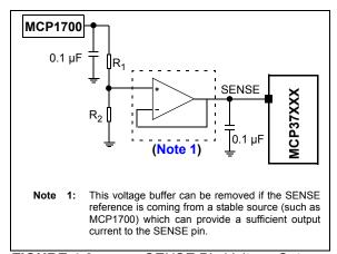
FIGURE 4-6: SENSE Pin Voltage Setup.
