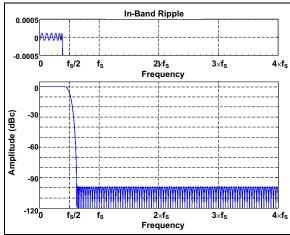
FIGURE 4-14: Response of the Octal-Channel Fractional Delay Recovery (1<sup>st</sup> Nyquist Band). f<sub>S</sub> is the Sampling Frequency.
