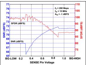
**FIGURE 3-34:** SNR/SFDR vs. SENSE Pin Voltage:  $f_S = 200$  Msps,  $f_{IN} = 15$  MHz.
