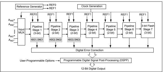
FIGURE 4-1: ADC Core Block Diagram.
