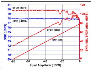
**FIGURE 3-26:** SNR/SFDR vs. Analog Input Amplitude:  $f_S = 200$  Msps,  $f_{IN} = 15$  MHz, High-Reference Mode (SENSE =  $AV_{DD12}$ ) with NSR enabled.  $A_{IN} \le 0.8$  dBFS for NSR.
