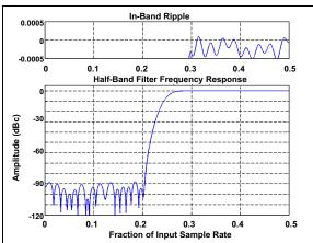
FIGURE 4-20: High-Pass (HP) Response of Half-Band Filter.
