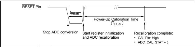
FIGURE 2-6: RESET Pin Timing Diagram.
