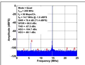
**FIGURE 3-8:** FFT for 14.7 MHz Input Signal:  $f_S = 50$  Msps/Ch., Quad,  $A_{IN} = -1$  dBFS.
