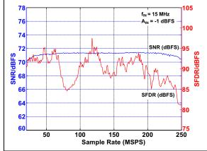
**FIGURE 3-33:** SNR/SFDR vs. Sample Rate (Msps):  $f_{IN} = 15$  MHz.
