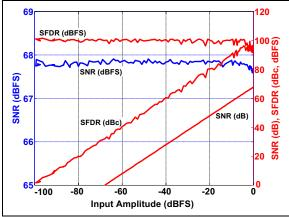
**FIGURE 3-28:** SNR/SFDR vs. Analog Input Amplitude:  $f_S = 200 \text{ Msps}$ ,  $f_{IN} = 70 \text{ MHz}$ , Low-Reference Mode (SENSE = GND).
