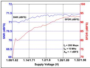
FIGURE 3-35: SNR/SFDR vs. Supply Voltage:  $f_S = 200 \text{ Msps}$ ,  $f_{IN} = 15 \text{ MHz}$ .
