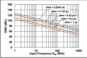
FIGURE 4-10: SNR vs. Clock Jitter.
