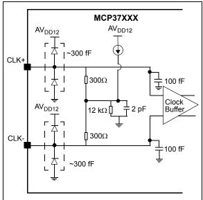
FIGURE 4-8: Equivalent Clock Input Circuit.
