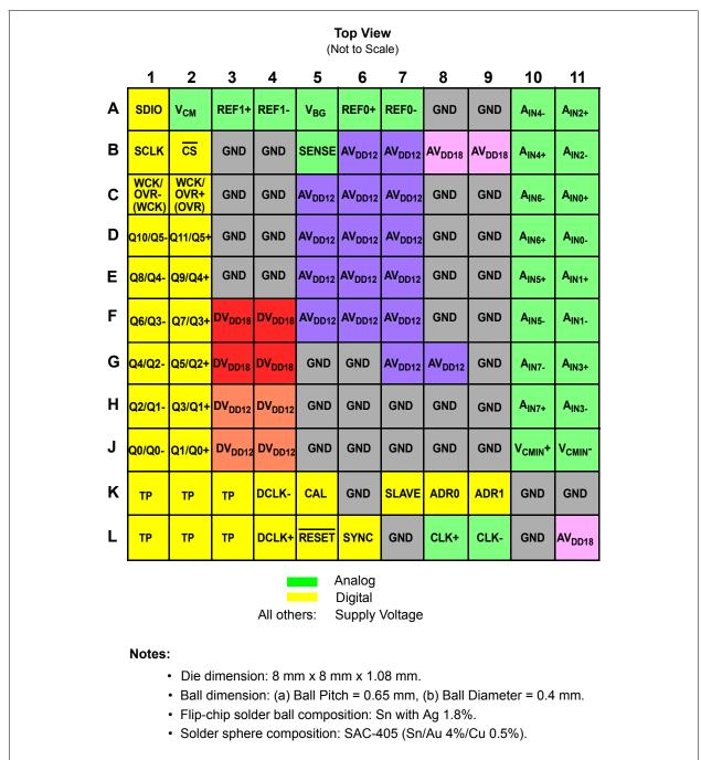
**FIGURE 1-2:** TFBGA-121 Package. See <u>Table 1-2</u> for the pin descriptions. Decoupling capacitors for reference pins and  $V_{BG}$  are embedded in the package. Leave TP pins floating always.
