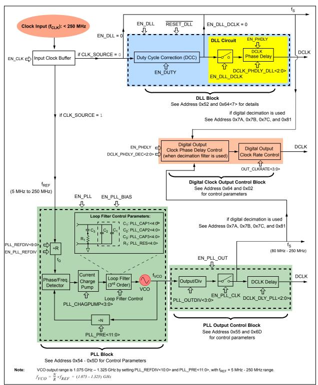
FIGURE 4-11: Timing Clock Control Blocks.
