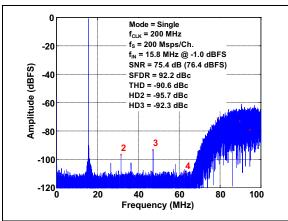
FIGURE 3-20: FFT for 15.8 MHz Input Signal with NSR enabled: NSR = 63,  $f_S = 200 \text{ Msps/Ch.}$ ,  $A_{IN} = -1 \text{ dBFS.}$
