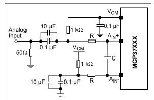
FIGURE 4-5: Singled-Ended Input Configuration.
