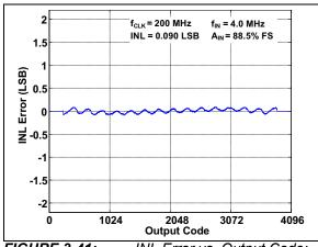
**FIGURE 3-41:** INL Error vs. Output Code:  $f_S = 200$  Msps,  $f_{IN} = 4$  MHz.
