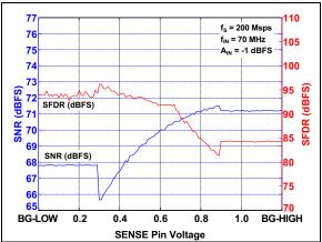
**FIGURE 3-31:** SNR/SFDR vs. SENSE Pin Voltage:  $f_S = 200 \text{ Msps}$ ,  $f_{IN} = 70 \text{ MHz}$ .
