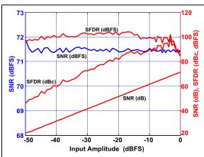
**FIGURE 3-24:** SNR/SFDR vs. Analog Input Amplitude:  $f_S = 200 \text{ Msps}$ ,  $f_{IN} = 15 \text{ MHz}$ , High-Reference Mode (SENSE =  $AV_{DD12}$ ).
