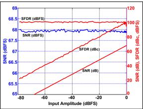
**FIGURE 3-25:** SNR/SFDR vs. Analog Input Amplitude:  $f_S = 200 \text{ Msps}$ ,  $f_{IN} = 15 \text{ MHz}$ , Low-Reference Mode (SENSE = GND).
