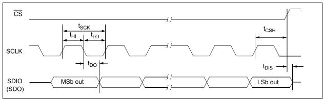
FIGURE 2-4: SPI Serial Output Timing Diagram.
