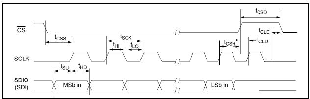
FIGURE 2-3: SPI Serial Input Timing Diagram.
