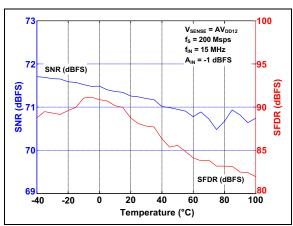
**FIGURE 3-36:** SNR/SFDR vs. Temperature:  $f_S = 200$  Msps,  $f_{IN} = 15$  MHz.
