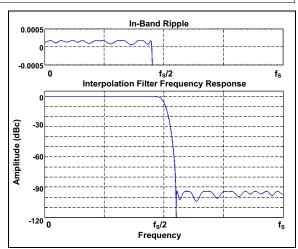
**FIGURE 4-13:** Response of the Dual-Channel Fractional Delay Recovery (1<sup>st</sup> Nyquist Band). f<sub>S</sub> is the Sampling Frequency.
