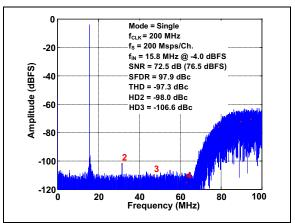
FIGURE 3-23: FFT for 15.8 MHz Input Signal with NSR enabled: NSR = 63,  $f_S = 200 \text{ Msps/Ch.}$ ,  $A_{IN} = -4 \text{ dBFS.}$
