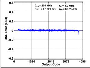
**FIGURE 3-42:** DNL Error vs. Output Code:  $f_S = 200 \text{ Msps}, f_{IN} = 4 \text{ MHz}.$
