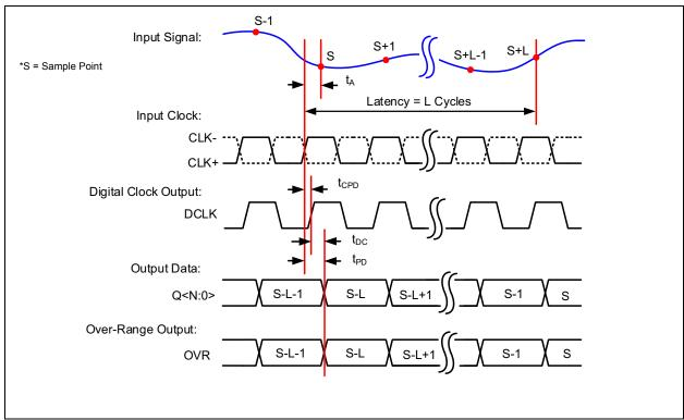
FIGURE 2-1: Timing Diagram - CMOS Output.
