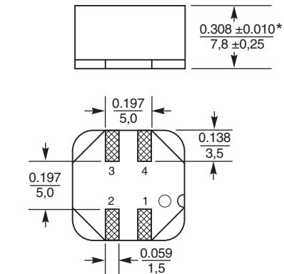
\* For optional tin-lead and tin-silver-copper terminations, dimensions are for the mounted part. Dimensions before mounting can be an additional 0.012 inch (0,3 mm).
