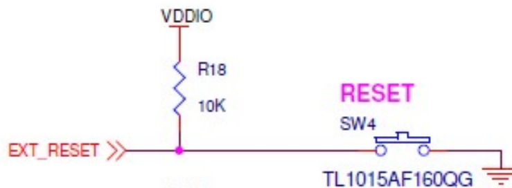
Figure 10. Using EXT_RESET pin
