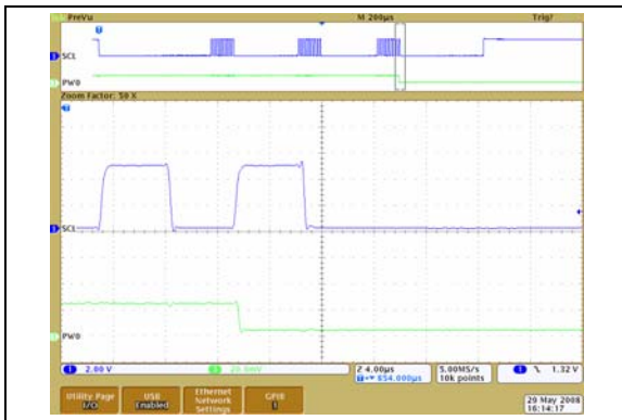
FIGURE 2-49: 50\text{ k}\Omega – Low-Voltage Decrement Wiper Settling Time ( V_{DD} = 5.5\text{V} ) ( 1\ \mu\text{s}/\text{Div} ).
