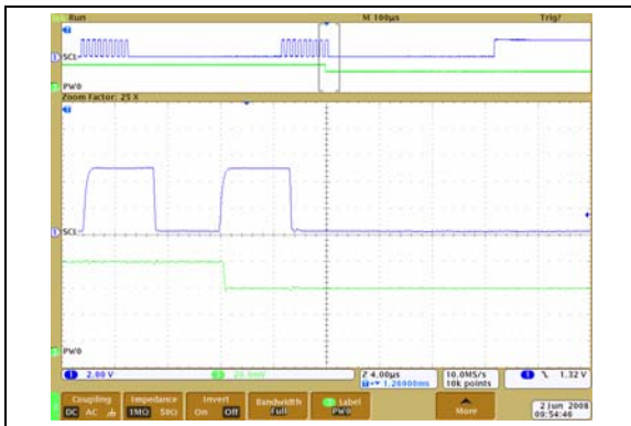
FIGURE 2-18: 5\text{ k}\Omega – Low-Voltage Decrement Wiper Settling Time ( V_{DD} = 5.5\text{V} ) ( 1\ \mu\text{s}/\text{Div} ).
