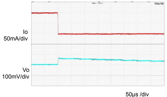
Figure 13. Transient Response ( T_a=105^\circ\text{C} ) ( I_o = 0.1\text{A} \rightarrow 0\text{A} )
