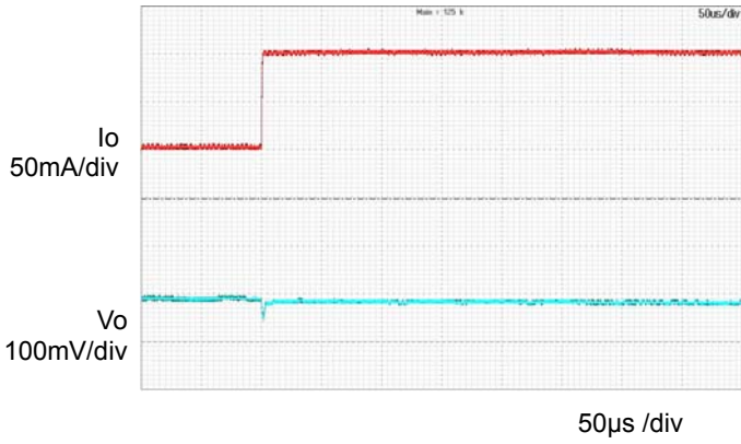
Figure 10. Transient Response ( T_a=-40^\circ\text{C} ) ( I_o = 0\text{A} \rightarrow 0.1\text{A} )
